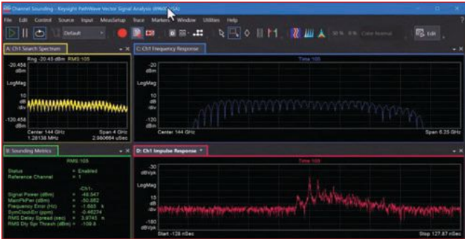
▲ Fig. 3 Channel sounding results portrayed by the 89600 VSA software in both frequency and time domains.
